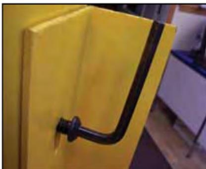
Tighten bolt with 5/16" allen key.
