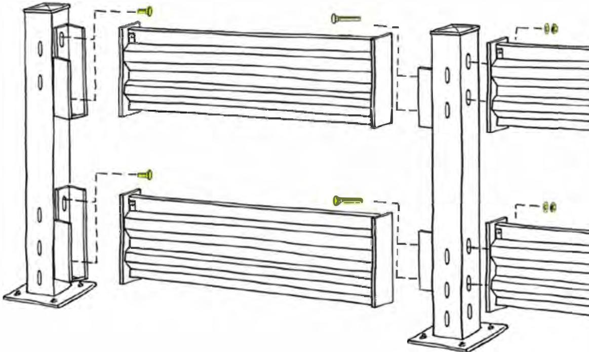
**NOTE:** Special fasteners are used when lift-out brackets are on each side of post or when lift-out bracket is mounted to end of post in guardrail run.
